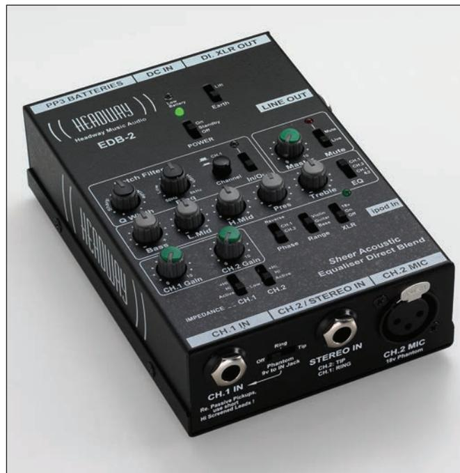
tuner output, and an aux/iPod in socket on 3.5 mm mini-jack (someone must find that useful...). The unit has a thread in the base for attaching a mic stand bracket if you want the controls within easy reach à la Martin Carthy or Steve Knightley.
